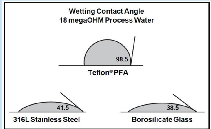
The data of table in the end of page indicate that PFA coating is more than 156% less wettable than glass, and more than 137% less wettable than electropolished 316L stainless steel.
